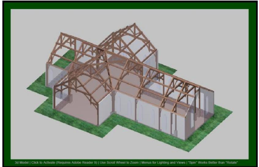
*Drawing featuring the new truss structure by Vermont Timber Work, Inc.*
